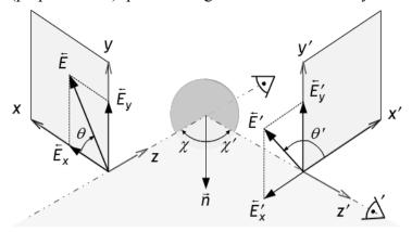
Fig. 8 Reflection of a Stokes vector.
