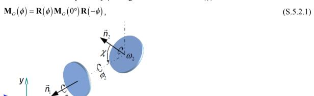
Figure 10 Rotation angles of an optical element. The rotations considered in this work are only  $\phi_1$  and  $\phi_2$ .
